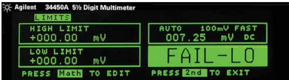
Figure 5. The display of 34450A in limit operation.
