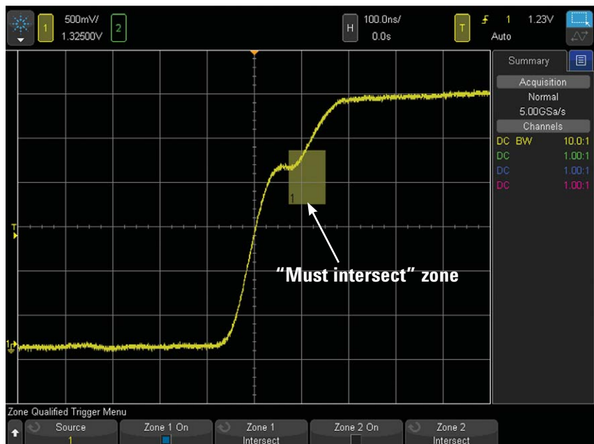
Figure 2: Capturing and displaying just waveforms with an anomaly (non-monotonic edge) using InfiniiScan Zone Trigger.
