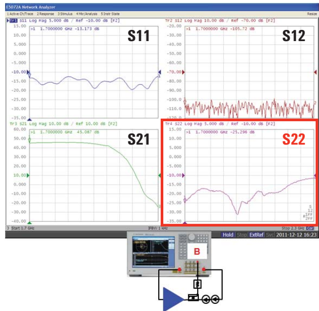
Figure 5. Measurement result of a high-power amplifier with a configuration using direct receiver access.
