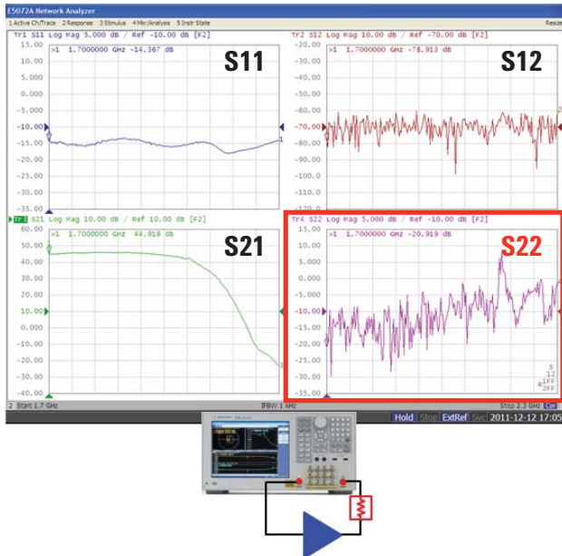
Figure 4. Measurement result of a high-power amplifier with a typical configuration with large attenuation.
