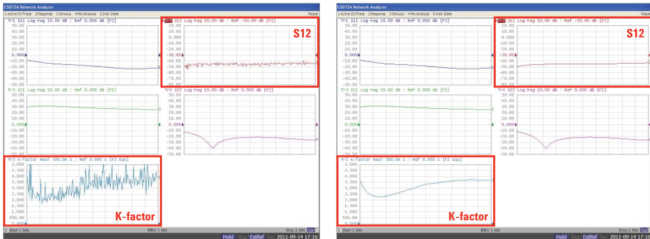
Figure 3. Comparison of K-factor results with coupled (left) and uncoupled (right) port power.
