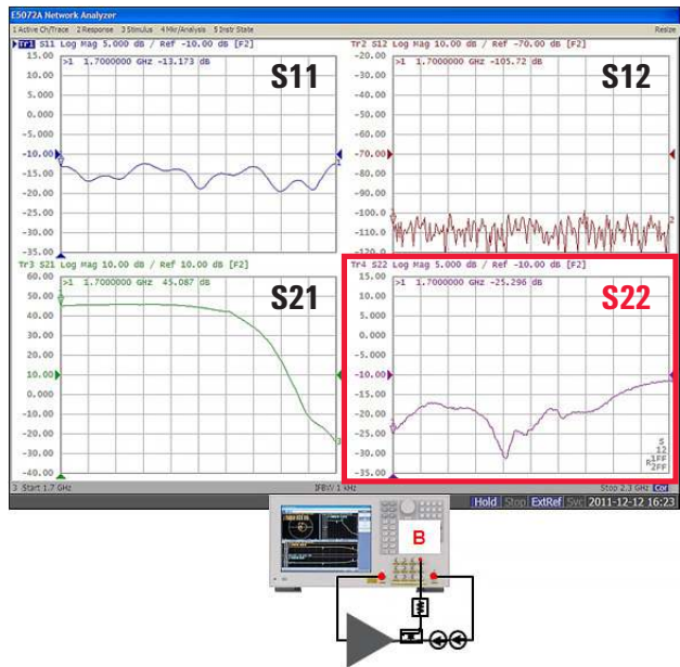
Figure 5. Measurement result of a high-power amplifier with a configuration using direct receiver access.
