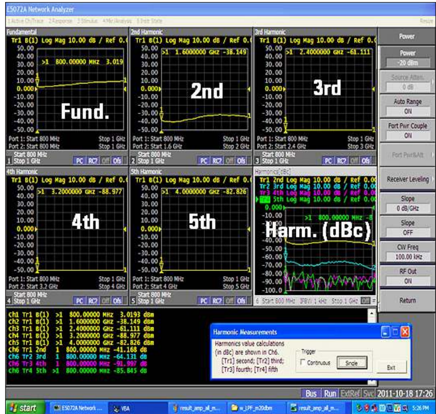
Figure 23. Measurement example of swept harmonic measurement with amplifier measurement wizard.
