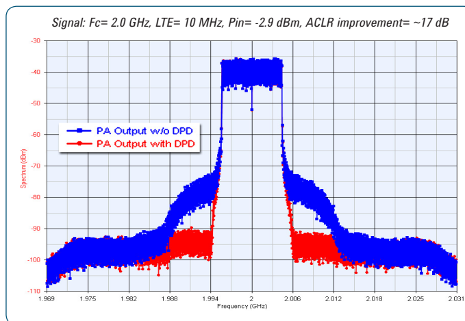
FIGURE 5: This example DPD extraction takes place at RF power = -2.9 dBm. The original raw data is displayed in blue, while the DPD+PA output is shown in red.
