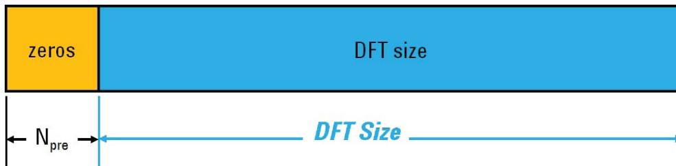
Figure 3(b) Payload OFDM symbol with zeros prefix
