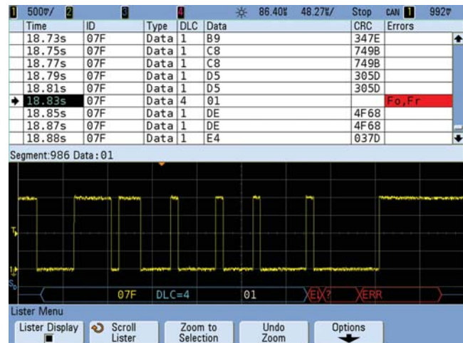
Figure 5: Capturing 1000 consecutive occurrences of just data frame ID: 07F.
