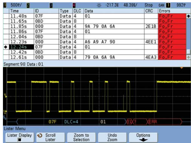
Figure 6: Capturing 100 consecutive occurrences of CAN error frames reveals a glitch in frame ID: 07F.
