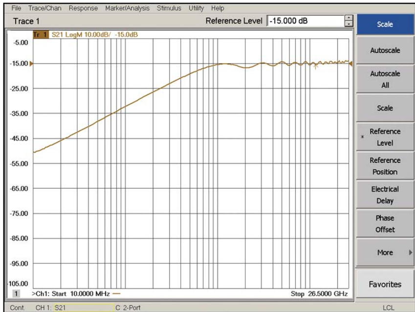
Figure 31. Test-port coupler frequency response (coupled arm)
