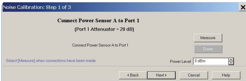
Figure 48. When using a power meter during calibration, the power level can be optimized independently from the channel power
