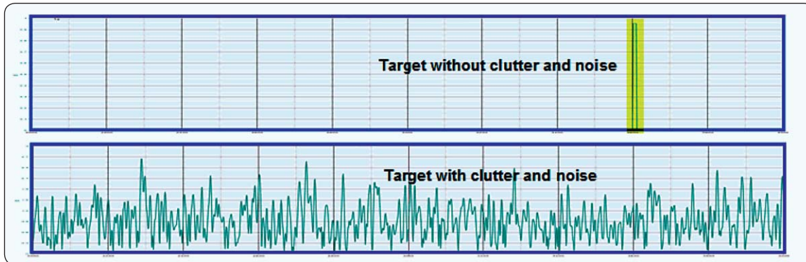
Figure 5-1. Target signal hidden by heavily cluttered environment
