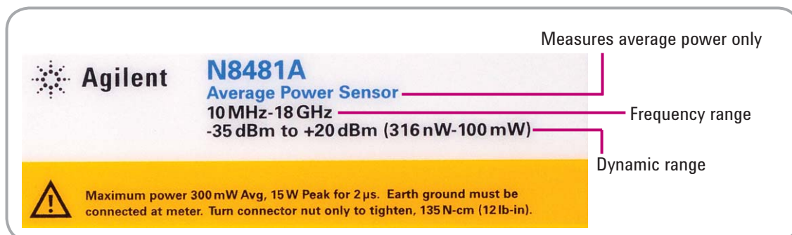
Figure 5. Front label of a thermocouple average power sensor
