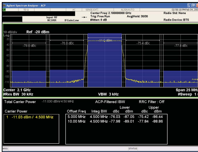
FIGURE 4: Typical adjacent channel power ratio performance with an MXG connected directly to an MXA.
