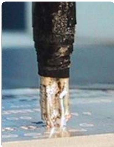
Figure 5. Close up of the custom, differential, semi-rigid coax probe tip.
