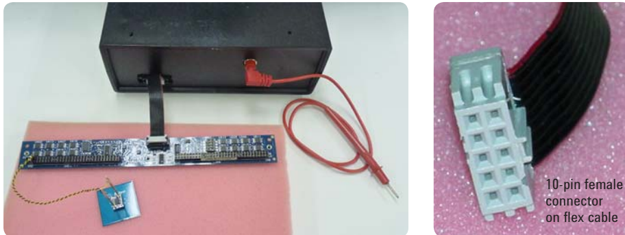
Figure 32. Flex cable connection
