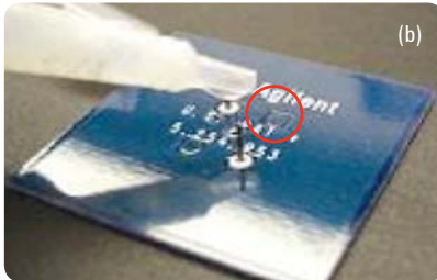
Figure 15. Apply adhesive (as denoted by the red circles)
