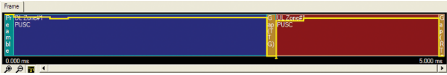
Figure 7. WiMAX TDD frame showing the DL with the preamble and PUSC zone, and the UL with a PUSC zone. The yellow trace shows power envelope
