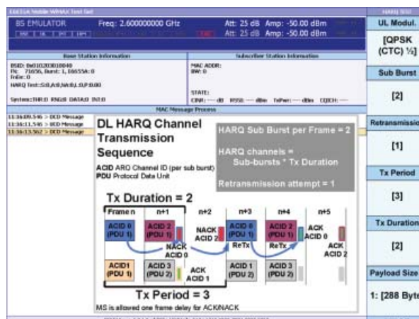
Figure 28. HARQ measurement as emulated using the E6651A test set
