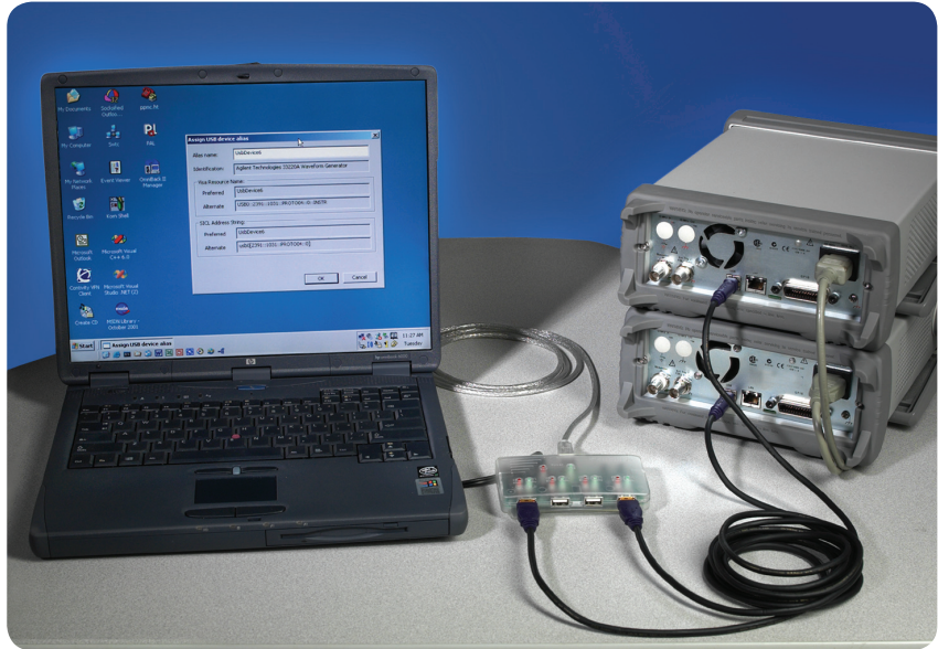
Figure 2. Using a USB hub with 2 USB instruments
