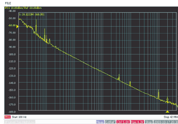
Figure 39. Bandwidth is limited to the bandwidth of the phase detector
