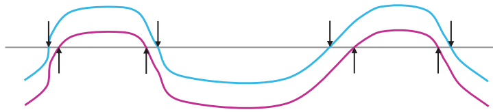
Figure 5. Example of how jitter can be caused by amplitude noise
