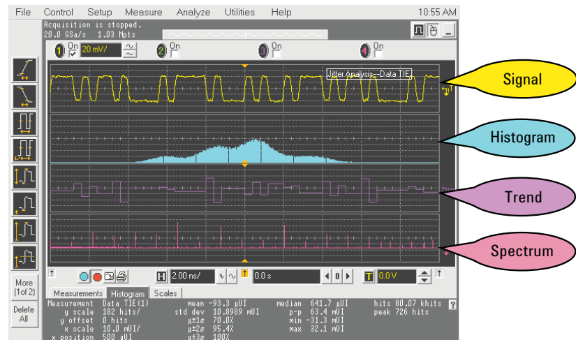
Figure 35. TIE analysis on a real-time oscilloscope
