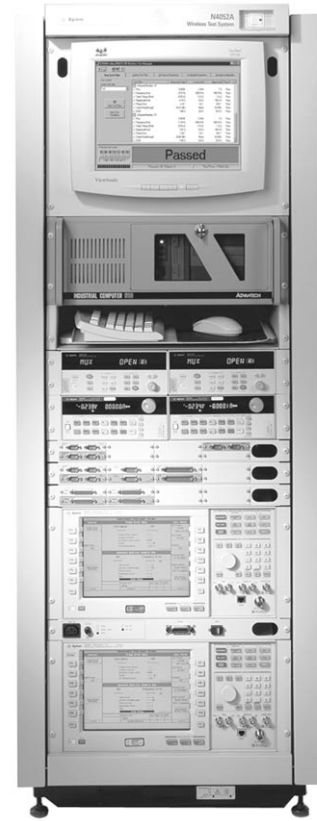
Figure 9.1. PC and test instruments in a rack
