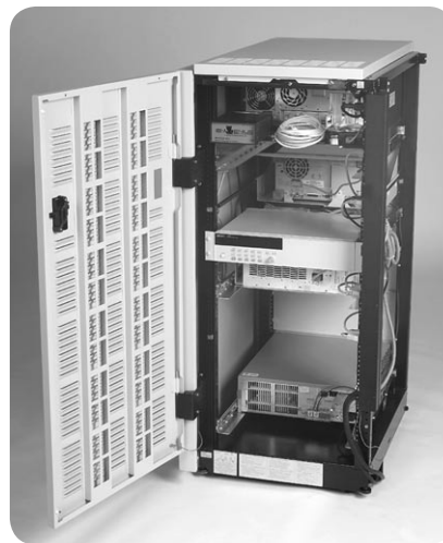
Figure 6.5. Rear-mounting the switching subsystem reduces rack space and minimizes cable lengths.
