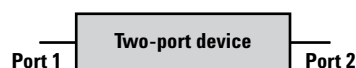
Figure 22.1. Modeling the RF signal path as a two-port device provides the S-parameters needed for calibration and correction.
