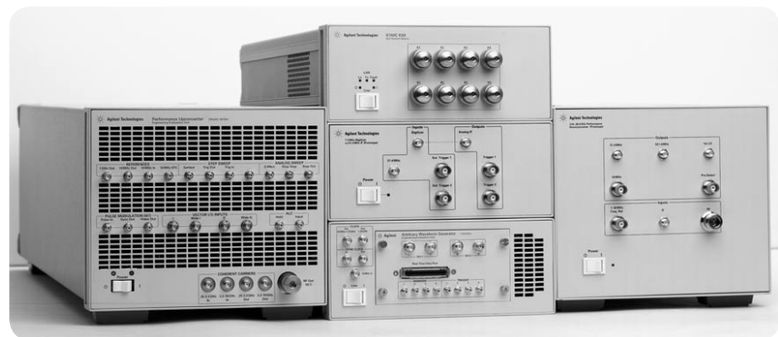
Figure 16.6. LXI devices reduce the size and footprint of test systems
