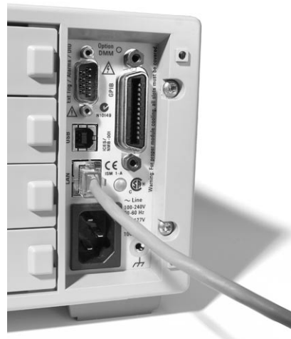
Figure 16.1. Current-generation instruments such as the Agilent 34980A switch/measure unit include LAN, USB and GPIB interfaces.
