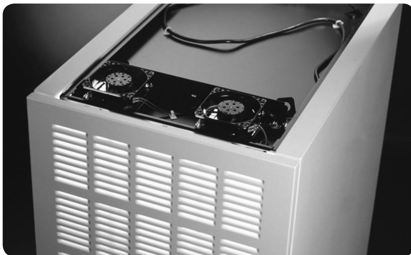
Figure 6.6. Extractor fan installed in rack
