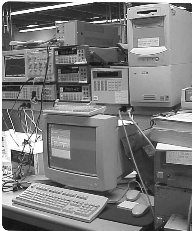
Figure 1.2. A test system using semi-automated control often uses a PC for the operator interface.
