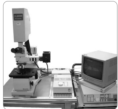
Figure 3. Scanning laser microscope used in subsurface measurement system.
