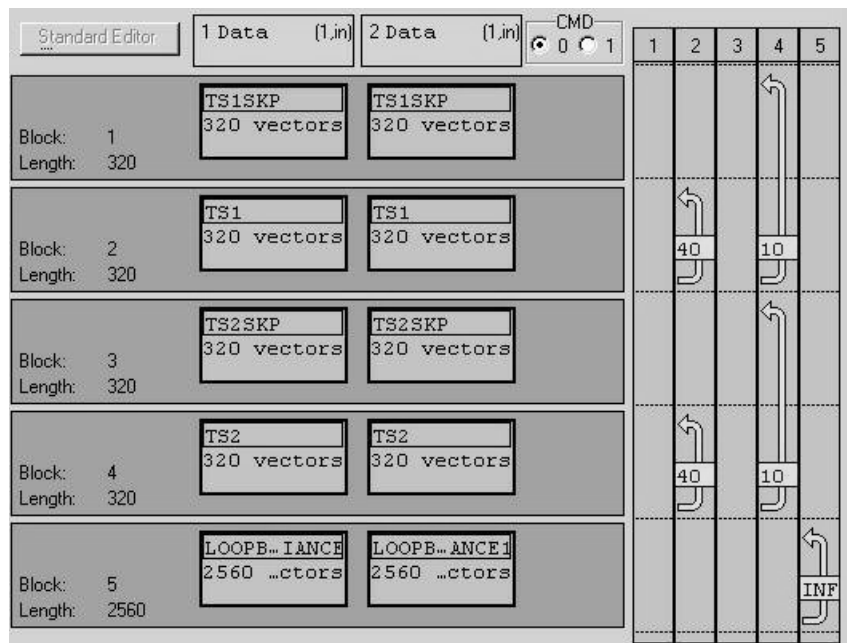
Figure 8: Nested Loop pattern for BER Measurement in Loop back
