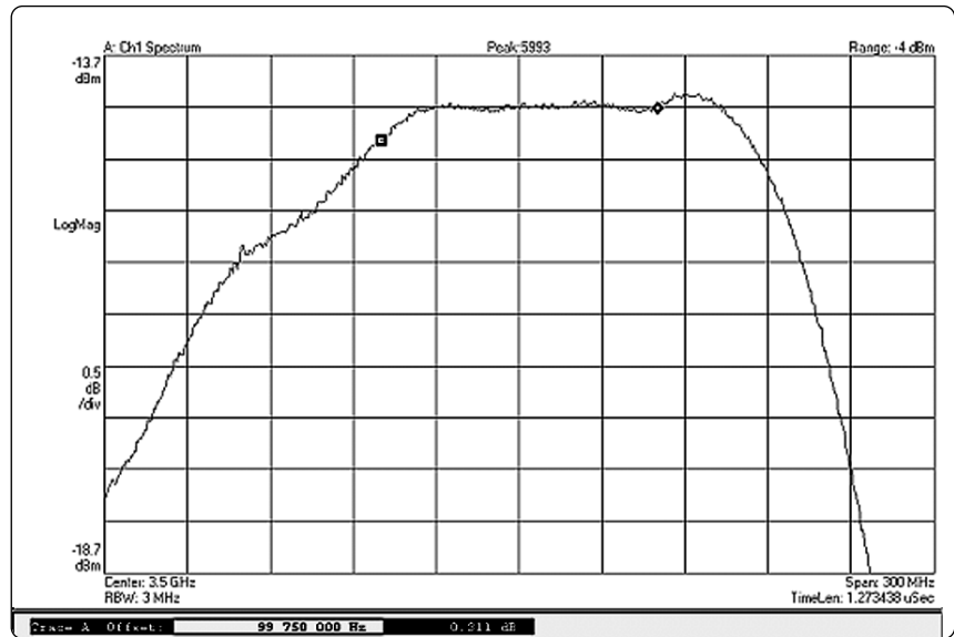
Figure 3. Un-corrected output from PSA Option HN8 showing 300 MHz wide span, with 0.5 dB per division
