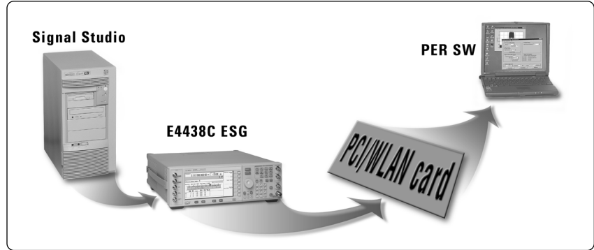
Figure 12: Setup for FER/PER using commercial sniffer software
