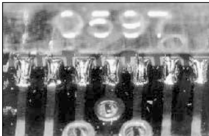
Figure 7.12 x-axis Misalignment Self-corrected after Reflow.
