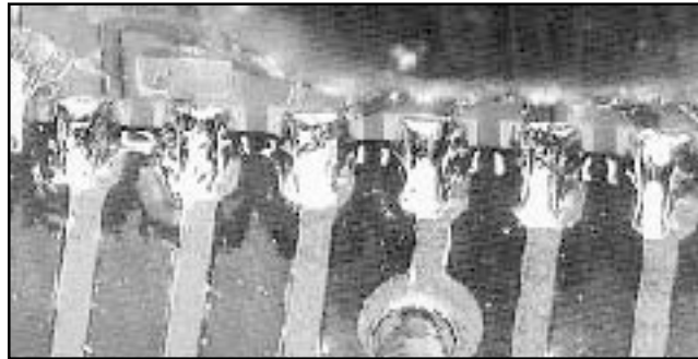
Figure 7.14 Good Solder Joint.
