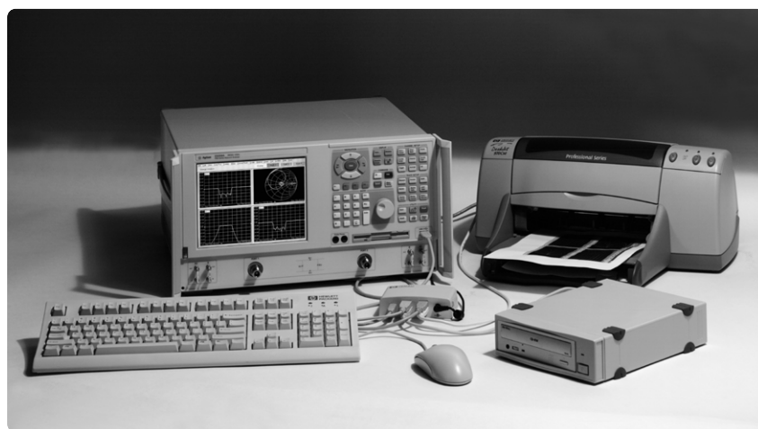
Figure 1. Agilent PNA Series network analyzers with LAN interface and Windows 2000
