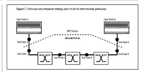
While stimulus-and-response testing has been used very successfully to test protocols, it can also be used to verify networks. This is one of the most important differences in the NewWAN testing paradigm. It has immediate benefits in terms of reproducing errors and setting known baselines to which the network can be compared at some point in the future. It establishes a pro-active approach towards problem resolution through active participation, rather than patiently awaiting the next failure.
